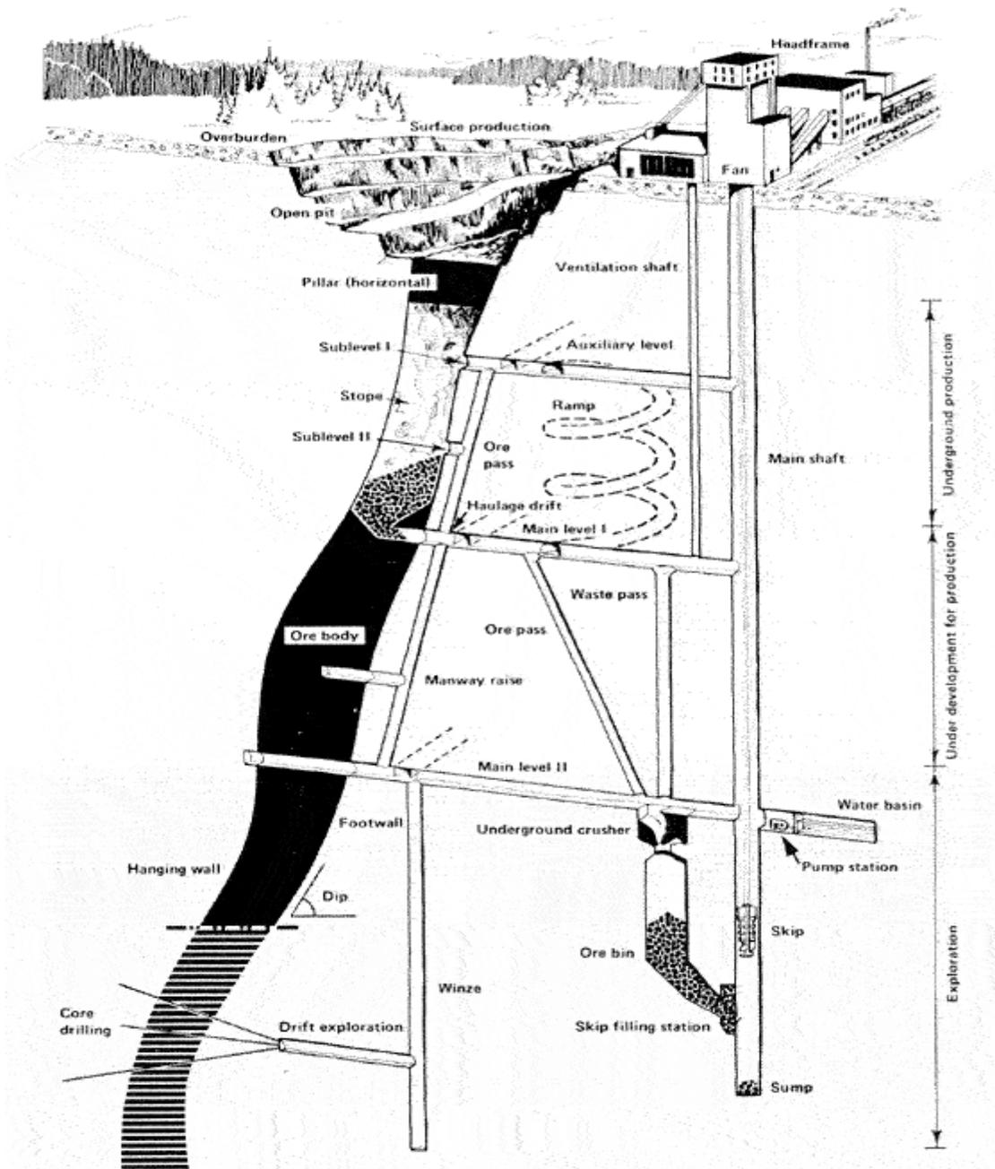
Fig. 1. Sample layout of an underground mine, identifying various mining operations and terms.
