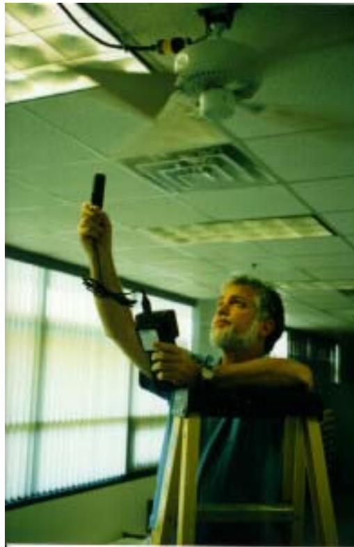
Figure 3. Operation of the prototype blades on a motor test assembly, showing Danny Parker measuring ceiling fan rotational speed (in rpm) using a hand-held Solomat infrared tachometer. (Source: Ref. 1.)
