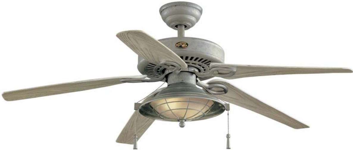
Figure 8. An indoor/outdoor version of the enhanced residential ceiling fan (the Gossamer Lighthouse model of the Gossamer Wind ceiling fan series). The fan has a decorative housing made of aluminum. The light is visible and the airfoil nature of the fan blades, including taper and twist, can be observed. (Source: Ref. 31.)
