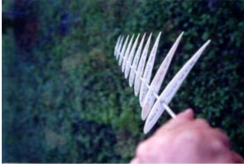
Figure 2. Partially completed prototype of the enhanced ceiling-fan blade, illustrating the airfoil profile as well as the varying blade twist and chord length with position along the blade. (Source: Ref. 1.)
