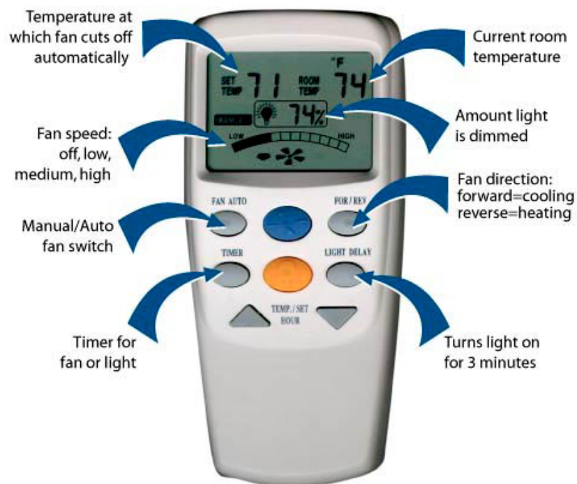
Figure 7. The hand-held remote control for the Gossamer Windward III ceiling fan, highlighting its control features. (Source: Ref. 31.)
